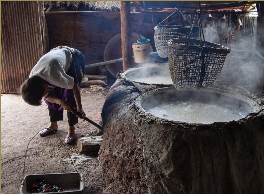
FIG. 1: OPEN PAN SALT MAKING IN BO KLUEA, THAILAND, WHERE WOOD IS USED AS FUEL. SALT WATER IS BEING BOILED TO REDUCE IT. THE SALT IS THEN PUT IN THE BASKETS AND SUSPENDED OVER THE PANS TO DRY IT OUT FURTHER. (CREDIT: TAKEAWAY / WIKIMEDIA)
