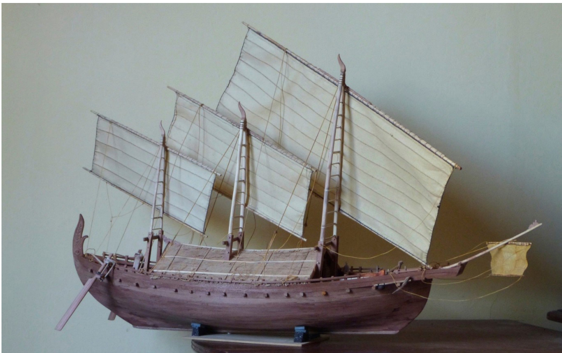
Fig. 61: A model of the 13th-century Java Sea Wreck , a Southeast Asian lashed-lug ship. (Courtesy of Nick Burningham)
