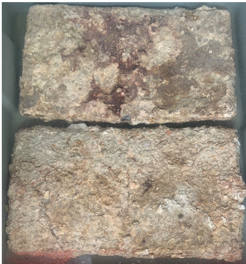
Fig. 23: Two intact tutenague ingots in sodium-sesquicarbonate solution.
