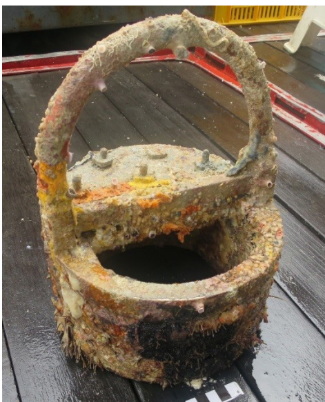
Fig. 52: A bilge pump valve with one flap missing.
