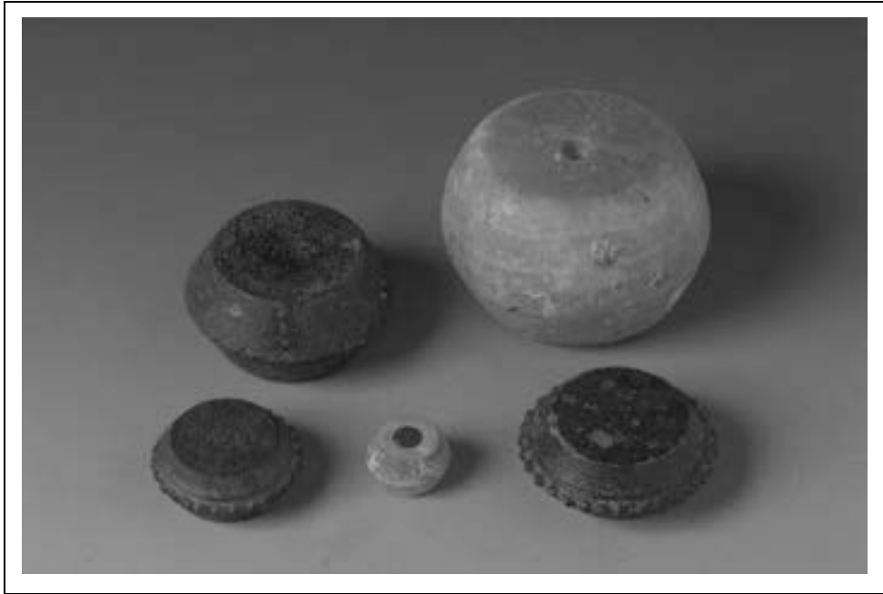
Different types of balance weights — plain Cu alloy (top left), scalloped Cu alloy (bottom left and right), composite (bottom center), and quartz (top right).
