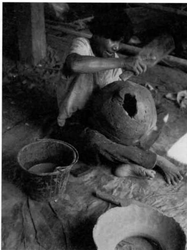
4. Potter closing base of pot using paddle and anvil. Baan Wang Tua, Khon Kaen Province, January 1995. Photo: Louise Cort.
