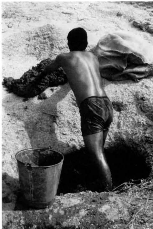
2. Man kneading rice husks and clay to make temper. Baan Wang Tua, Khon Kaen Province, January 1995. Photo: Louise Cort.
