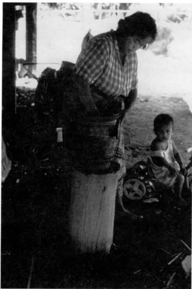
3. Potter shaping pot with paddle and anvil on post while walking forward around it. Baan Wang Tua, Khon Kaen Province, January 1995. Photo: Louise Cort.
