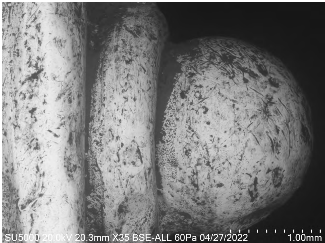
Fig. 21: SEM of a) surface of joints between bead, wire and plaque; b) at \times 300 magnification.
