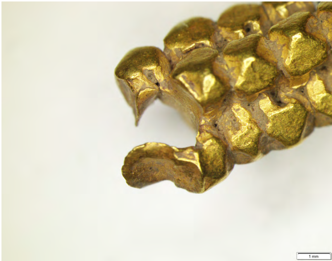
Fig. 12: Weathered edges of a ruptured bead.
