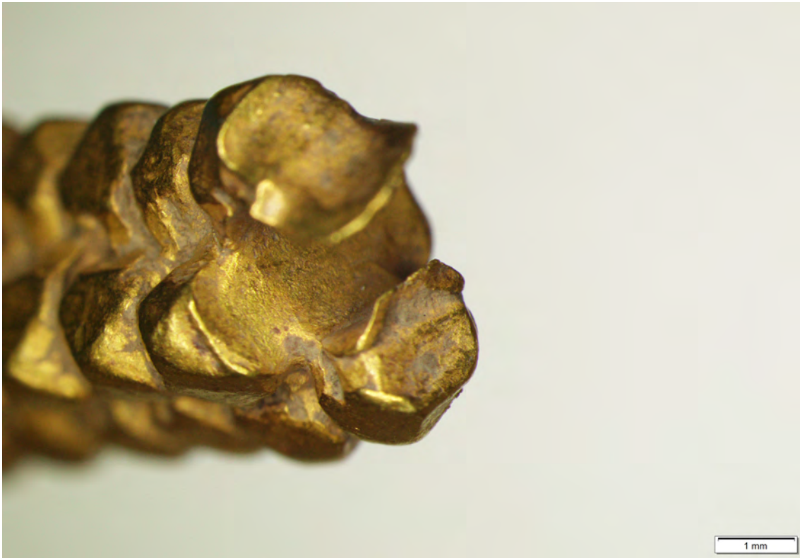
Fig. 11: Broken ends of two strands with ruptured bead.
