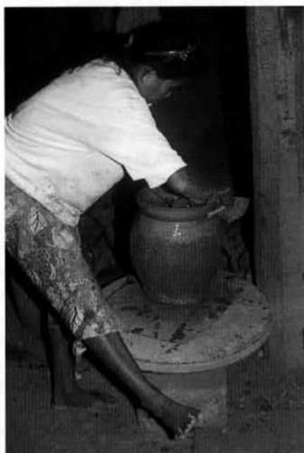
Fig. 1. Village A, potter shapes neck and rim of preform on fast wheel made from bicycle wheel.
