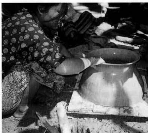
Fig. 2. Village B, potter shapes neck and rim of preform on board.
