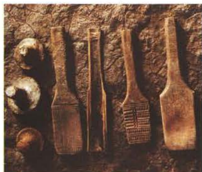
Figure 22 Set of tools (left to right): fired clay anvils; worn- out carved wooden pat- tern paddle; bamboo paddle; new carved wooden pattern paddle, with patterns for neck (upper left quadrant) and body (remaining three quadrants); plain wooden paddle. Vietnam, Kien Giang, Hon Dat, Sok Xoai, Dầu Doi, 1998.
